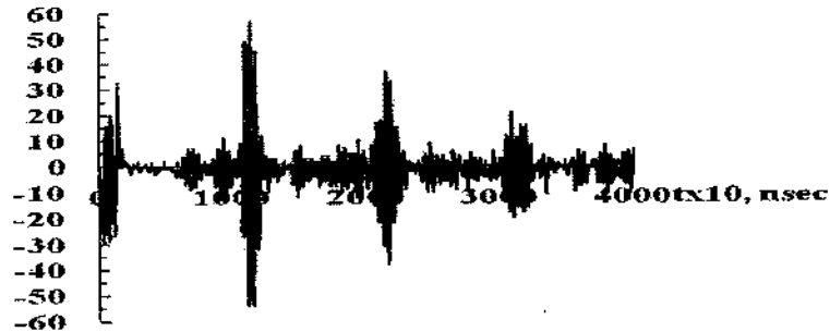
Fig. 4. Oscillogramma of impulses with transversal polarization, which are reflected in nanocomposite based on modify teflon-3M and MWCNT
