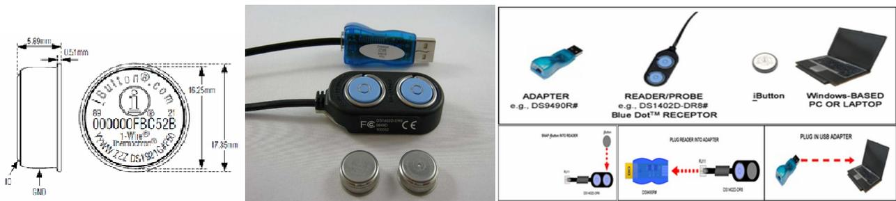
Fig. 2. Thermochron iButton DS1921G thermal sensors and schematic diagram of Blue Dot™ receptor & USB adapter
