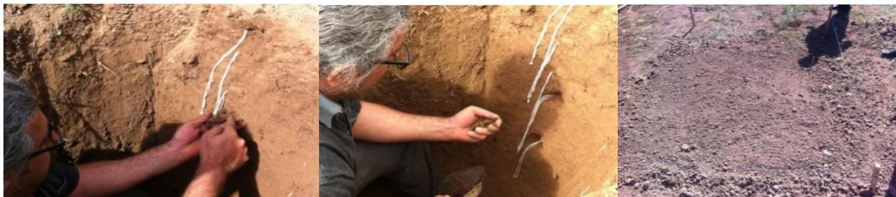
Fig. 3. Placing the thermal sensors in soil a profile
