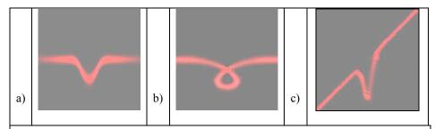
$\label{eq:Fig. 1} Fig.~1~Refractogramms~calculated~for~the~plane-structured~laser~radiation~propagated~through~:~a,~b-a~cylindrical~inhomogeneity,~c-plane~stratified~inhomogeneity$
