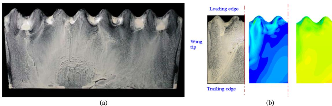
Fig. 1 (a) Flow visualization of a modified NACA 0012 airfoil with protuberances (aspect ratio of 2) at angle of attack 14 degree. Vortices between protuberances, separation behind protuberances, and tip vortices are clearly seen. (b) For NACA 0012 airfoil with protuberances (aspect ratio of 1) at angle of attack 30 degree, the separation bubble pattern shown by visualization (left) is consistent with vorticity (center) and pressure (right) distribution.
