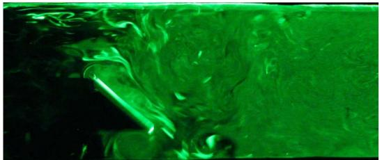
Fig. 2 Top view of duct flow with flapper towards the side
