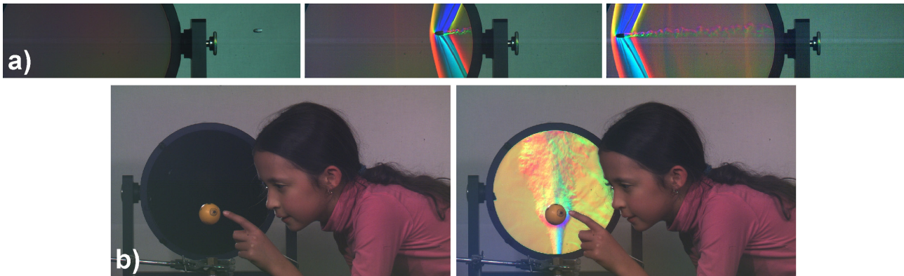
Fig. 7: Time-resolved images obtained with a coincident schlieren system (direction-indicating color schlieren), in which the area surrounding the schlieren field of view is simultaneously imaged.
