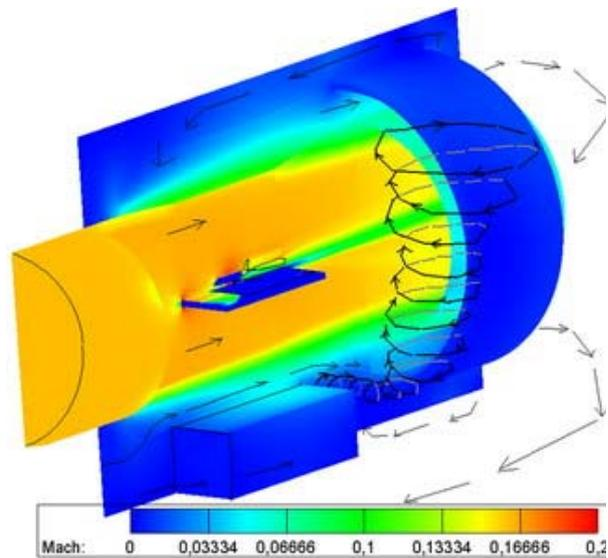
Fig. 3 Mach number field and restoration of streamlines in the test section of the T-104 wind tunnel.
