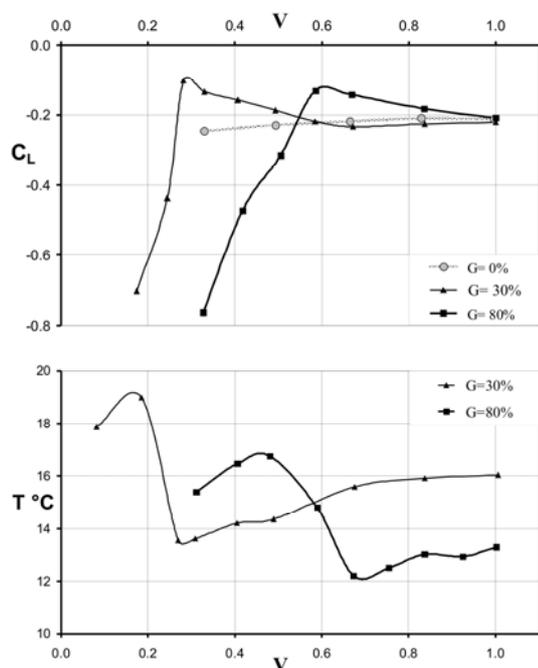
Fig. 4 The influence of rolling speed on the lift coefficient and the gas temperature at the air inlet
