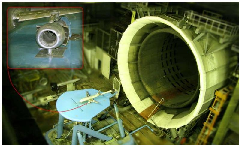
Fig. 1 Experimental setup in the T-104 wind tunnel
