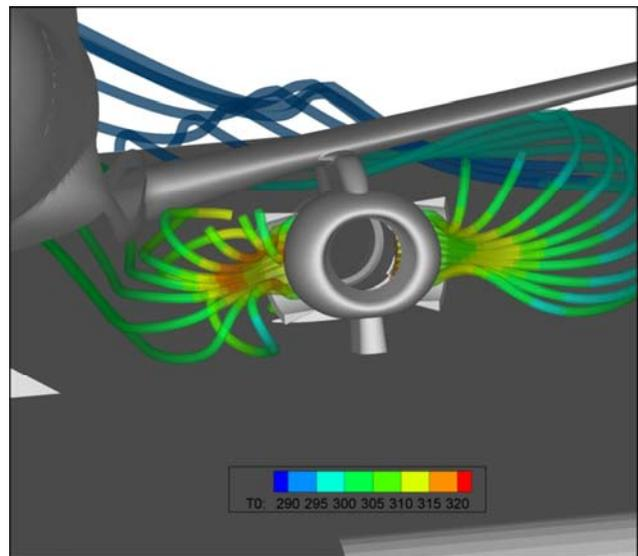
Fig. 9 Calculated stream filaments flowing out of the reverser
