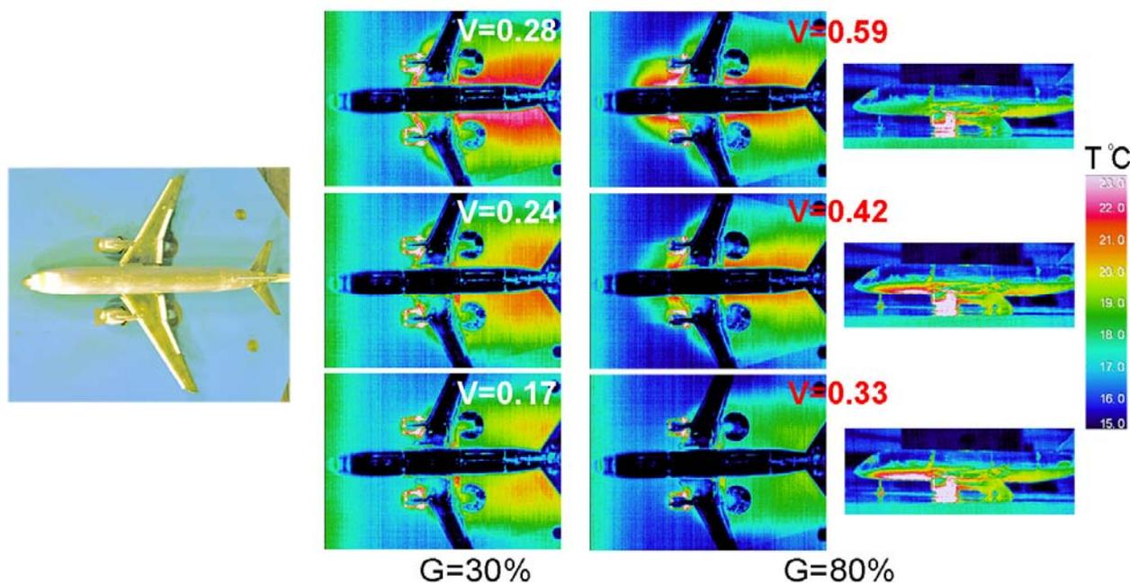
Fig.6 The effect of rolling speed on temperature field at  $G=30\%$  &  $G=80\%$  (visible model image and thermograms)
