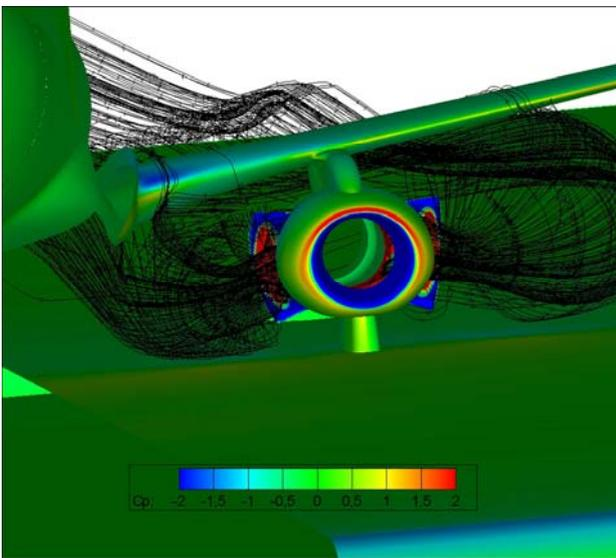
Fig.7 Calculated pressure coefficient field and streamlines in the engine's vicinity
