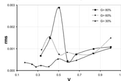
Fig.5 The effect of rolling speed on rms of the model's pitching angle.
