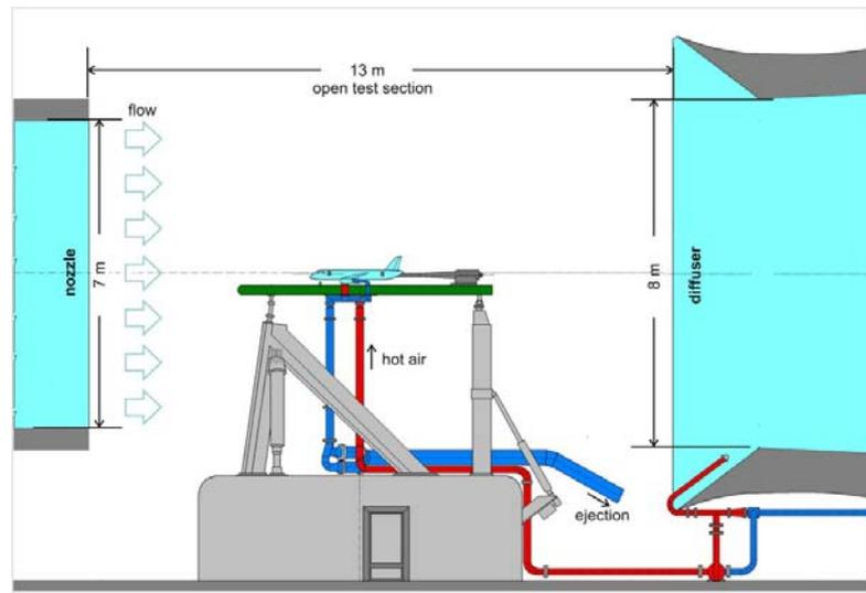
Fig. 2 Schematic of the thrust reversal setup
