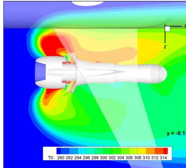
Fig. 10 Calculated temperature field at the  $Y=-0.145$  station
