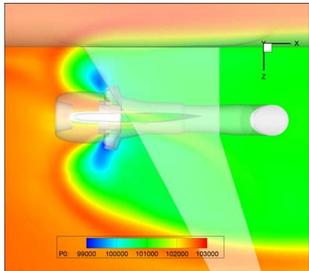
Fig. 8 Calculated total pressure distribution in the engine's vicinity
