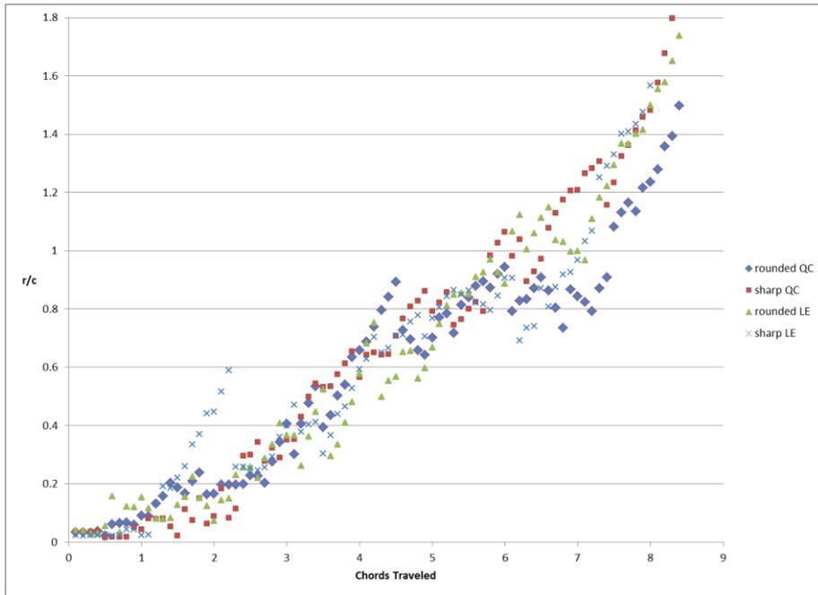
Fig. 8 Variation of the distance of the LEV core to the leading edge of the wing with respect to time when the mid-span location is illuminated for slow motion case
