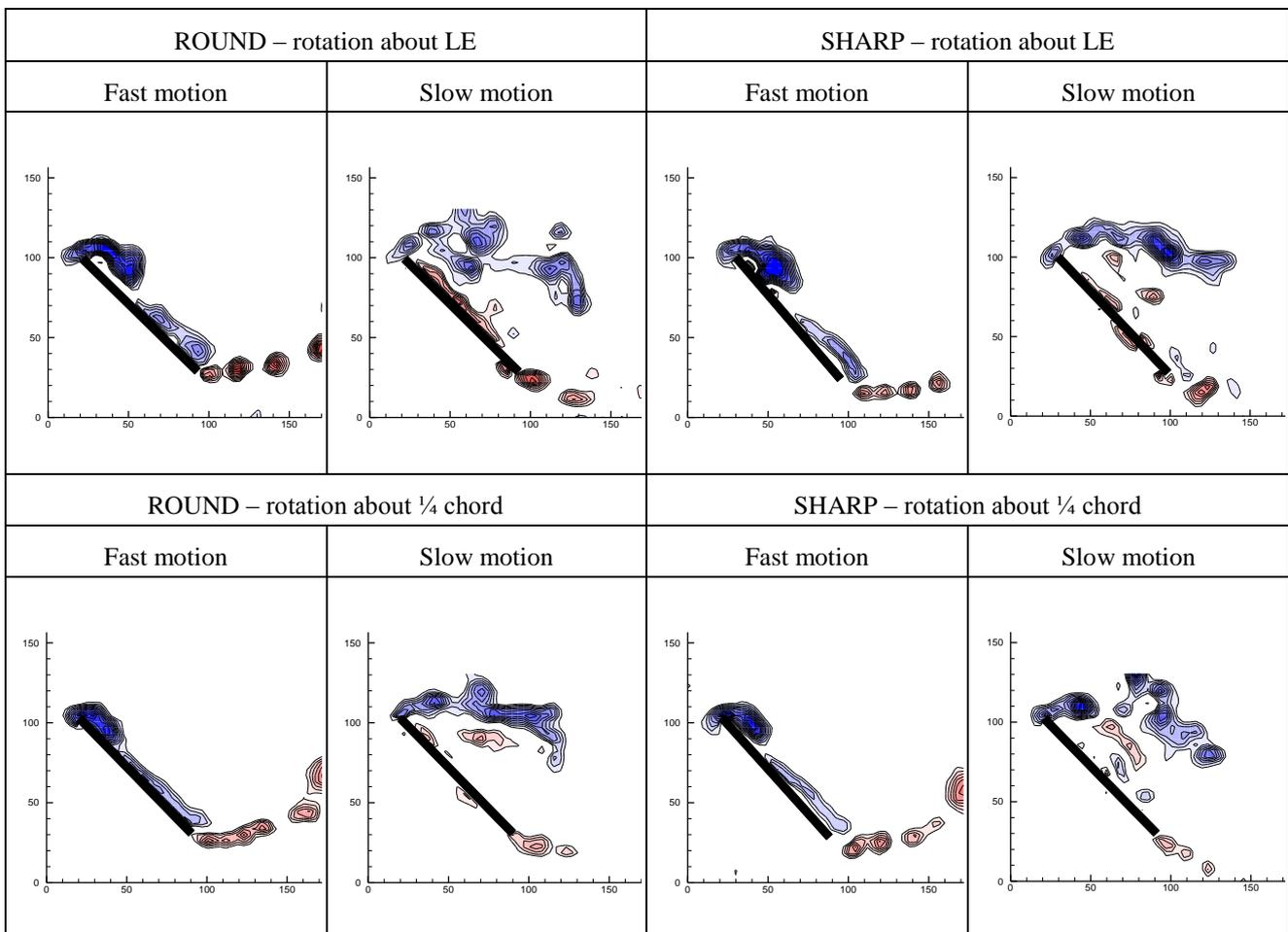
Fig. 4 Patterns of vorticity for thin rectangular plate when the mid-span location is illuminated
