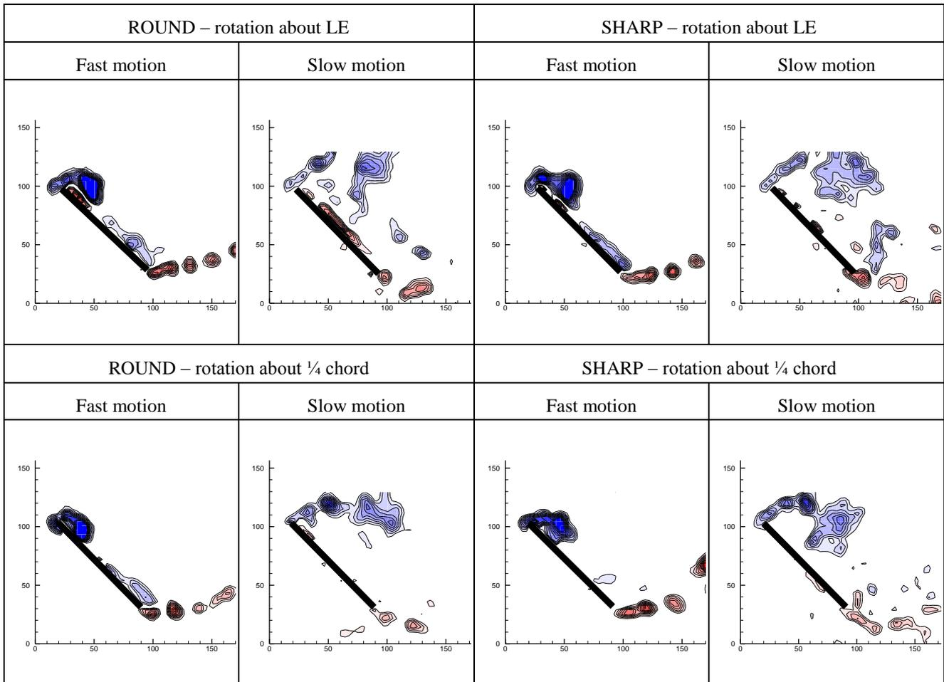
Fig. 5 Patterns of vorticity for thin rectangular plate when the quarter-span location is illuminated
