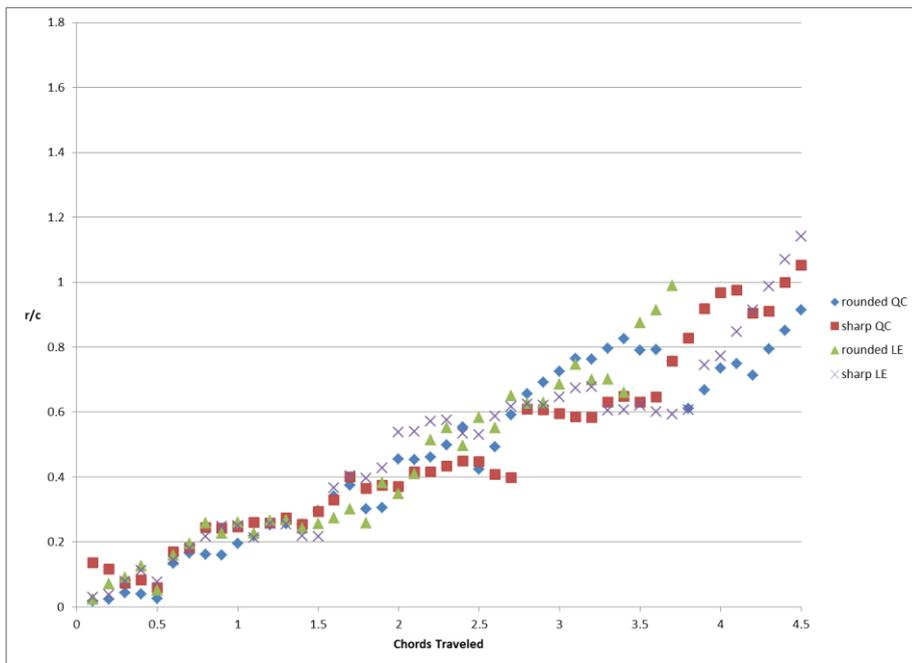
Fig. 7: Variation of the distance of the LEV core to the leading edge of the wing with respect to time when the quarter-span location is illuminated for fast motion case
