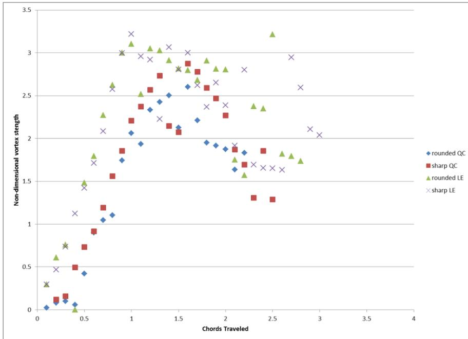
Fig. 10 Variation of the LEV strength with respect to time when the quarter-span location is illuminated for fast motion case
