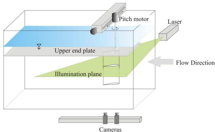
Fig. 2 Experimental setup showing the model and DPIV system
