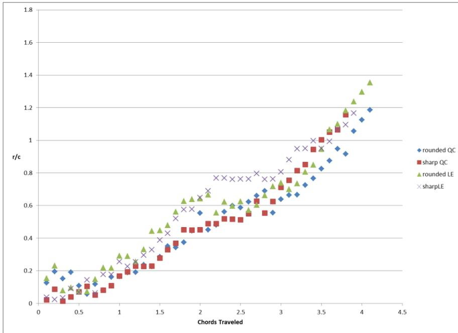
Fig. 6 Variation of the distance of the LEV core to the leading edge of the wing with respect to time when the mid-span location is illuminated for fast motion case
