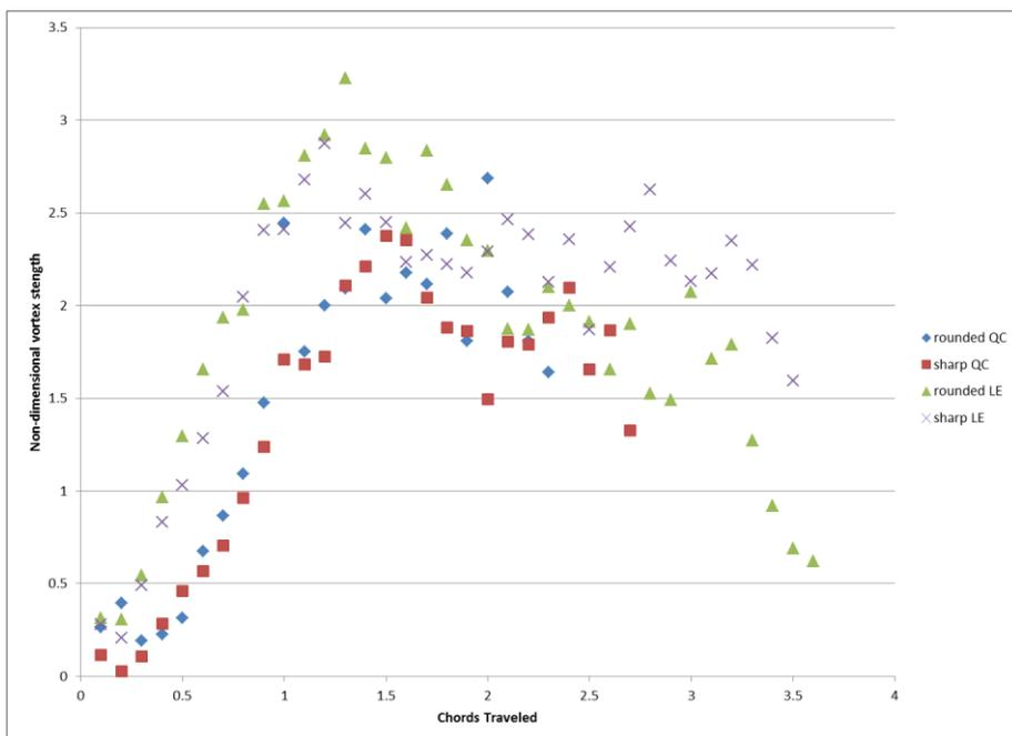
Fig. 9 Variation of the LEV strength with respect to time when the mid-span location is illuminated for fast motion case
