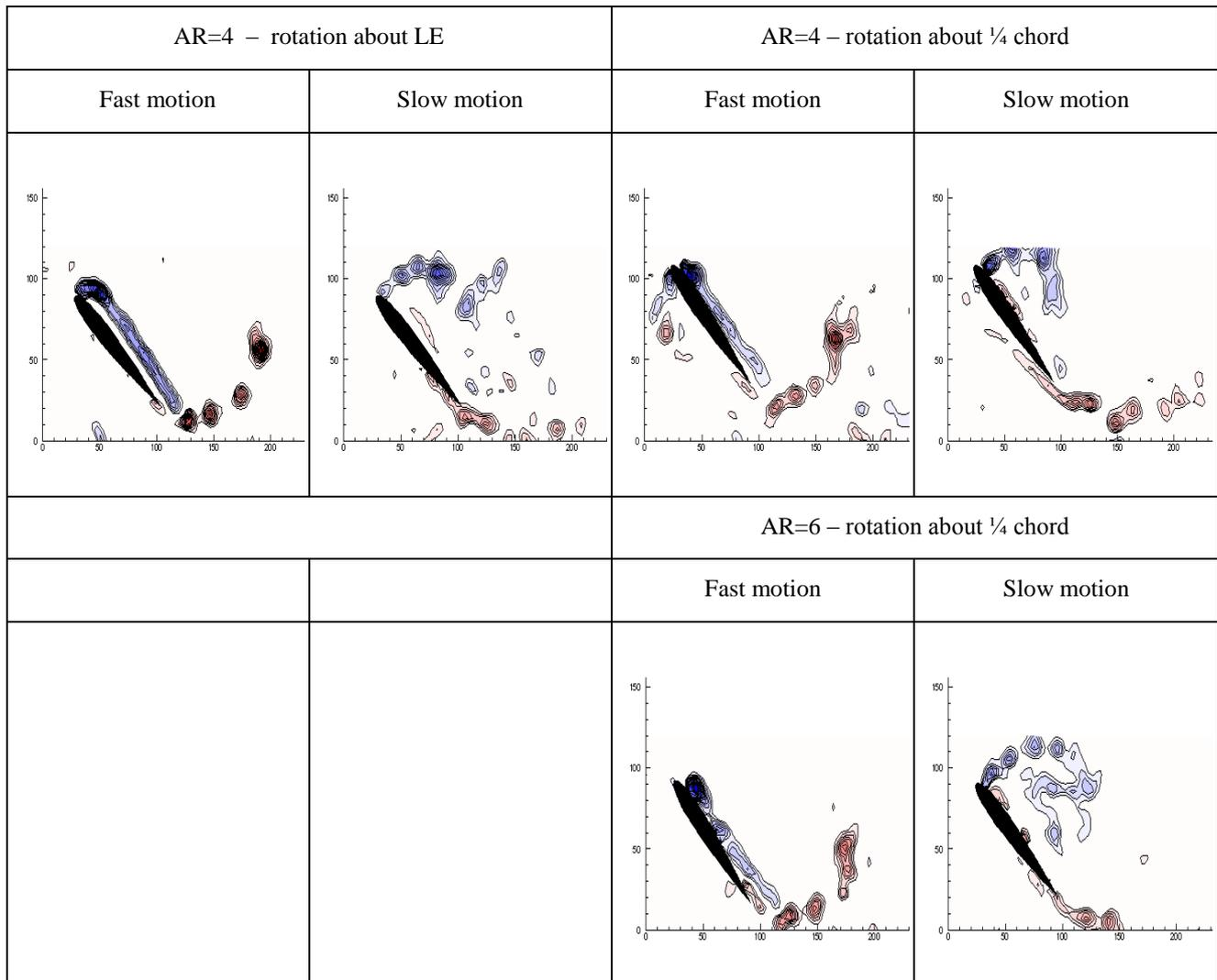
Figure 12: Patterns of vorticity for NACA0012 when the quarter-span location is illuminated
