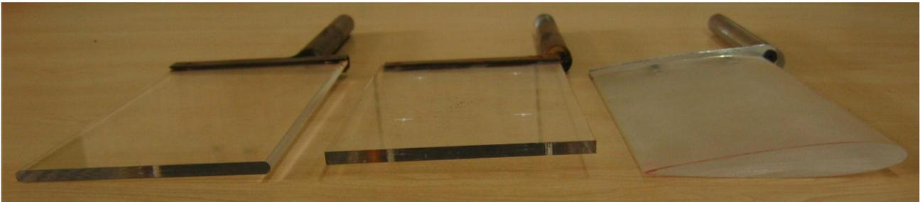
Fig. 1 The models used in the study, a NACA0012 airfoil and thin rectangular plates with round and sharp edges
