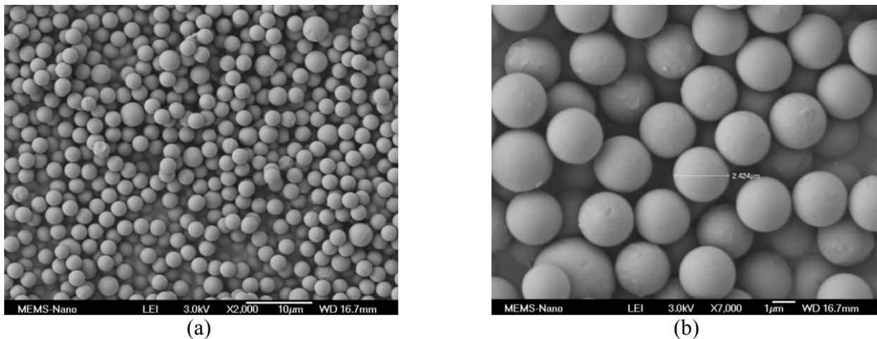
Fig. 1 SEM images of OSParticles fabricated by dispersion polymerization method (a) 2000X (b) 7000X.
