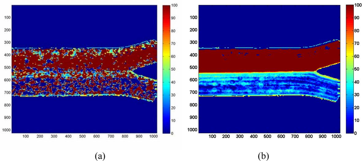
Fig. 7 (a) Instantaneous DO concentration field and (b) ensemble averaged DO concentration field
