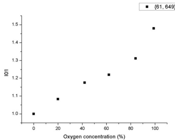
Fig. 5 Stern-Volmer plot at (61, 649) interrogation window
