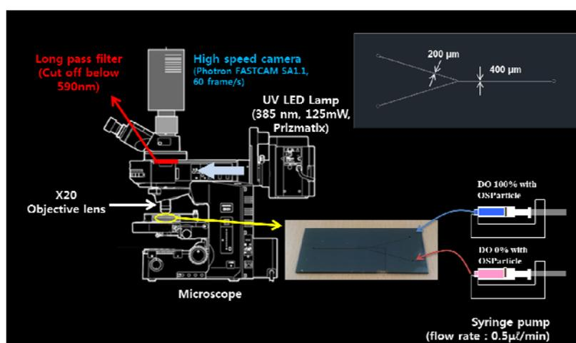
Fig. 3 Experimental setup for simultaneous measurement of DOC and velocity field in microchannel
