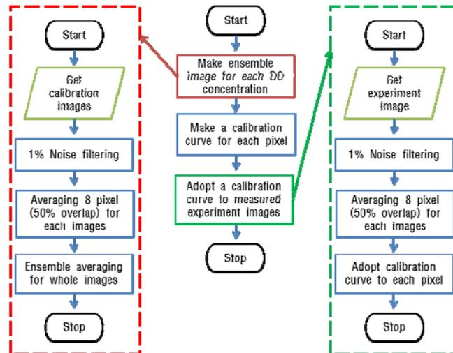
Fig. 4 The flow chart of modified pixel by pixel calibration procedure
