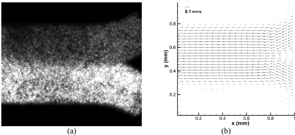
Fig. 6 (a) The Luminescence OSParticle image in microchannel and (b) ensemble averaged velocity vector field extracted from the OSParticle images
