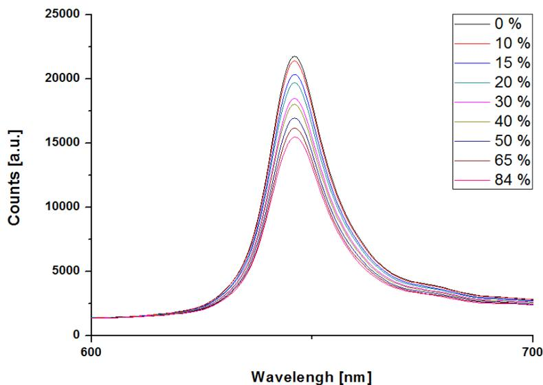
Fig. 2 The Variation of luminescent intensity by increasing DO concentration
