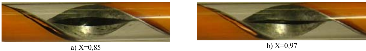
Fig. 7. Cord flows development in tube with twisted tape insert while change of gas content (liquid is colored in dark): G=7 g/s, p=0,13 MPa, S/d=3
