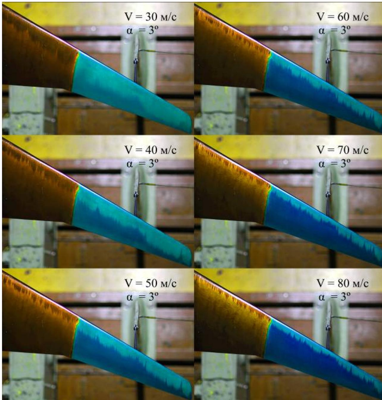
Fig. 2 Visualization of laminar-turbulent transition by shear stress sensitive liquid crystals at different flow velocities, angle of attack  $\alpha = 3^\circ$ , LC initialization along the flow
