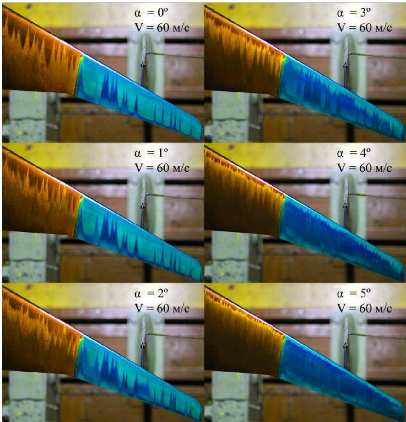
Fig.3 Visualization of laminar-turbulent transition by shear stress sensitive liquid crystals at different angles of attack, flow velocity  $V=60\text{m/s}$ , LC initialization across the flow
