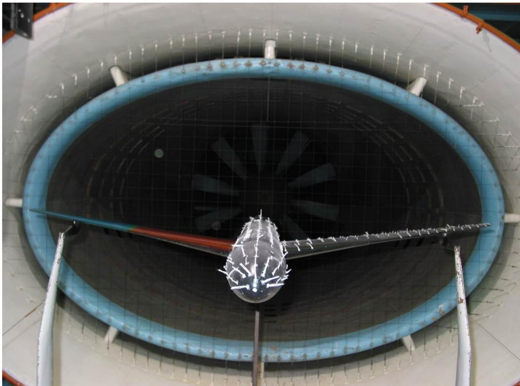
Fig. 1 Layout of the model in the T-103 test section
