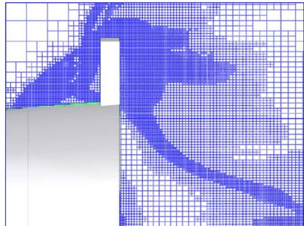
Fig. 2. An adapted mesh when flowing along model 5 with an initial velocity respective to  $M = 6$  after 4 rearrangement ( $N = 1700, 2550, 3400, 4250$  iterations) with formation of  $n = 2208346$  counting cells.
