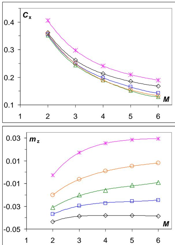
Fig. 7. Influence of a flow velocity on aerodynamic coefficients of model 2 for  $\alpha = -2, 0, 2, 5$  and  $10^\circ$  (rhomb, square, triangle, circle and  $\times$ ).
