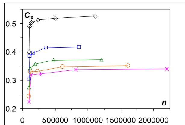
Fig. 3. Change of drag coefficients of model 1(left) and model 5 (right) when increasing the number of counting cells  $n$  for  $M = 2 - 6$  (rhomb, square, triangle, circle and ж).
