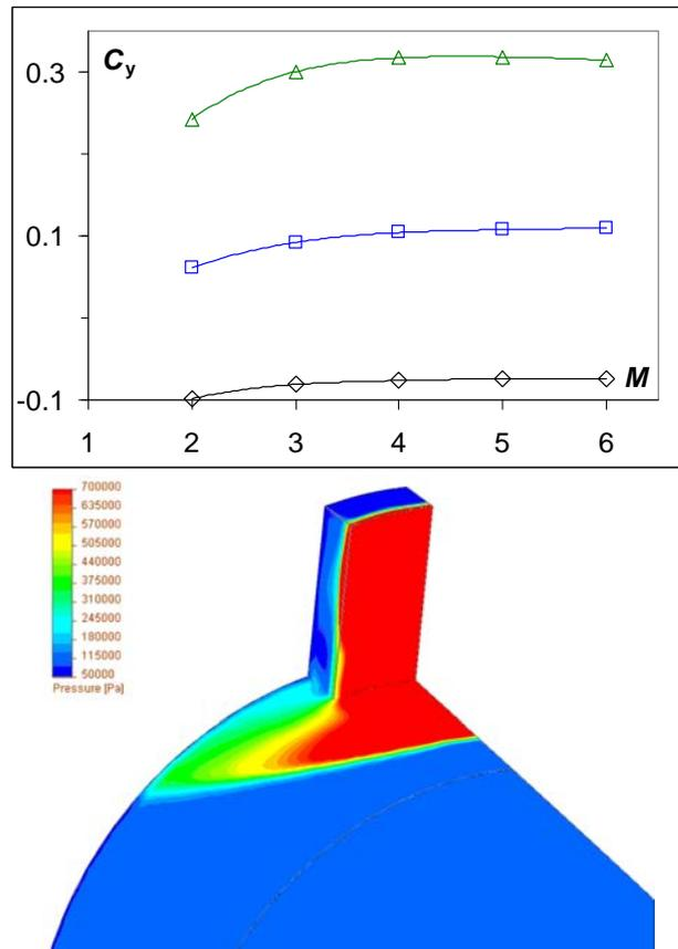
Fig. 11. Pressure distribution on the surface of model 3 near and on the control flap for  $\alpha = 0^\circ$  and  $M = 4$ .
