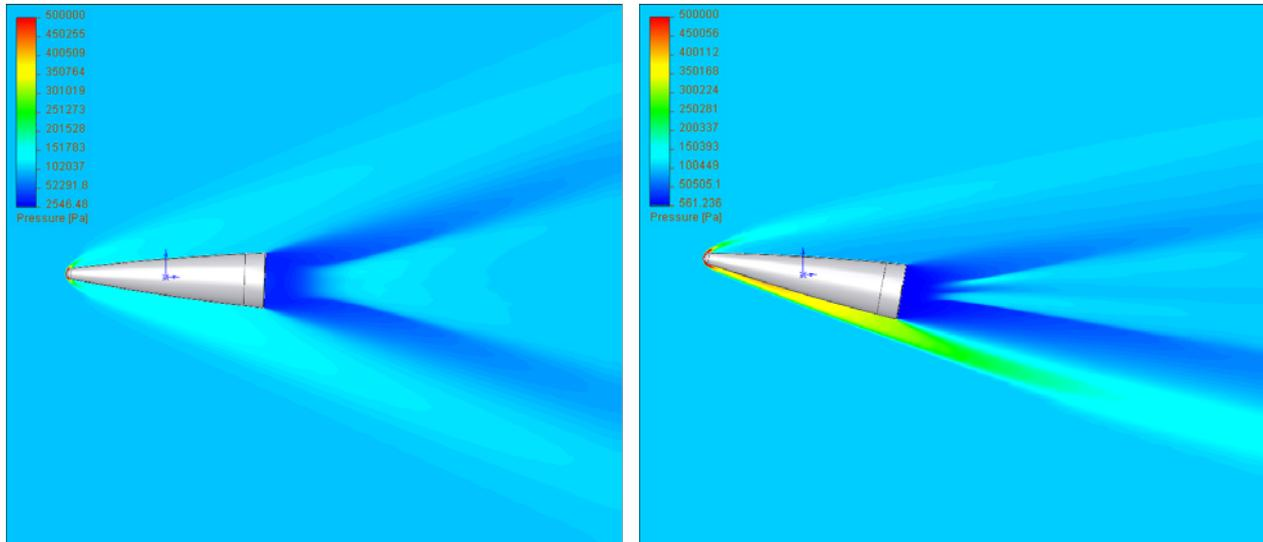
Fig. 4. Flow character of model 1 (pressure fields) for the cases when  $\alpha = 2^\circ$ ,  $M = 3$  (left) and  $\alpha = 10^\circ$ ,  $M = 5$  (right).
