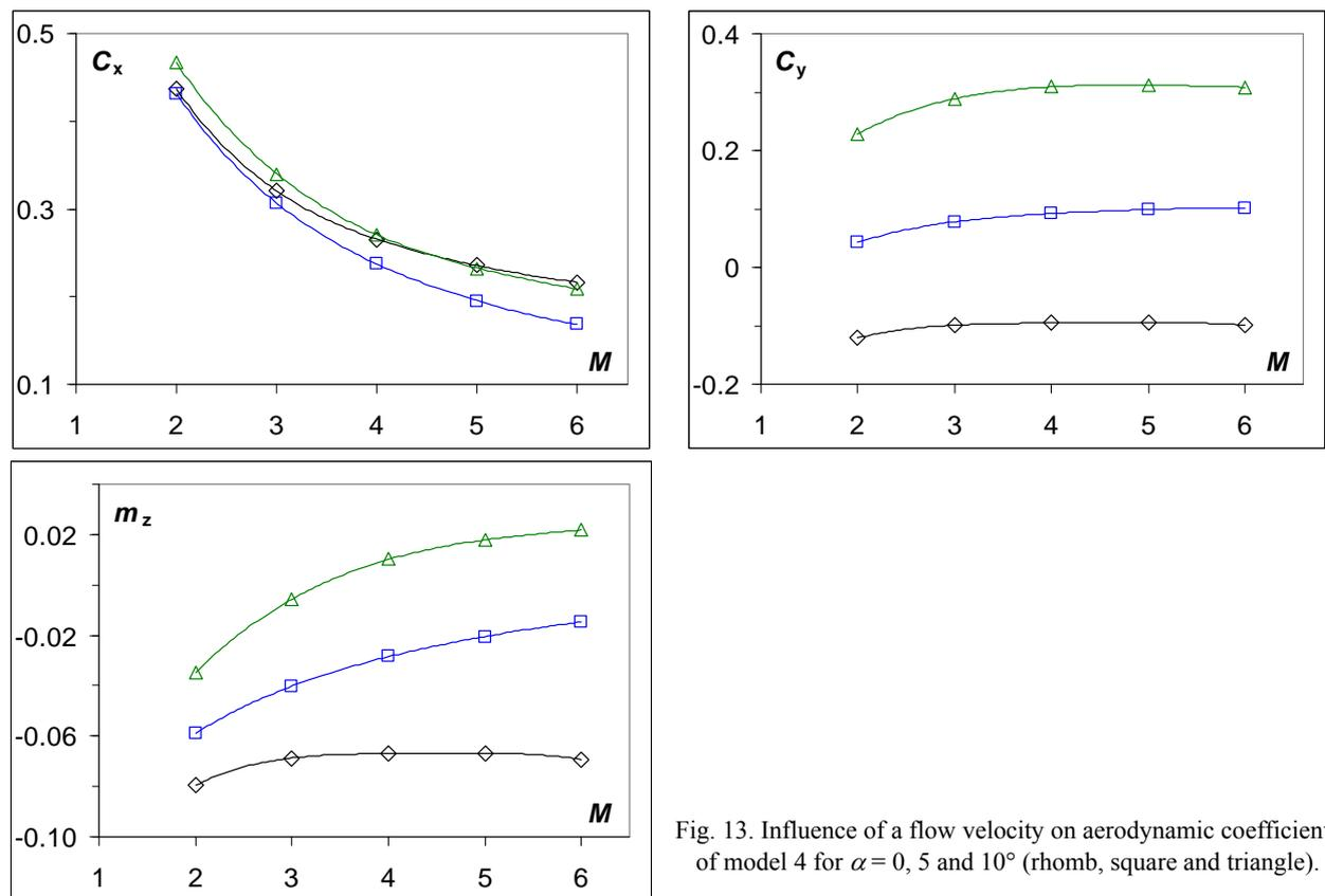
Fig. 13. Influence of a flow velocity on aerodynamic coefficients of model 4 for  $\alpha = 0, 5$  and  $10^\circ$  (rhomb, square and triangle).
