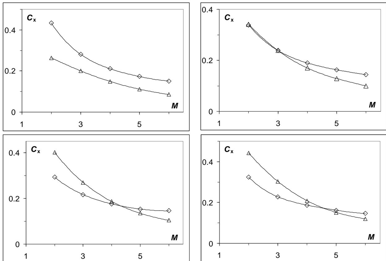
Fig. 20. Influence of a flow velocity on drag coefficients of the leader (rhomb) and block (triangle) situated at different distances ( $\Delta = 0, 0.5, 1, 1.5D$  – left to right, top to bottom) for  $M = 4$ .
