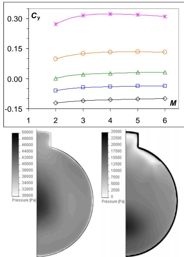
Fig. 8. Pressure distribution on the back surface of model 2 for  $M = 2$  (left),  $M = 6$  (right) and  $\alpha = 0^\circ$ .
