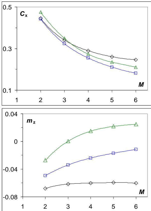
Fig. 10. Influence of a flow velocity on aerodynamic coefficients of model 3 for  $\alpha = 0, 5$  and  $10^\circ$  (rhomb, square and triangle).
