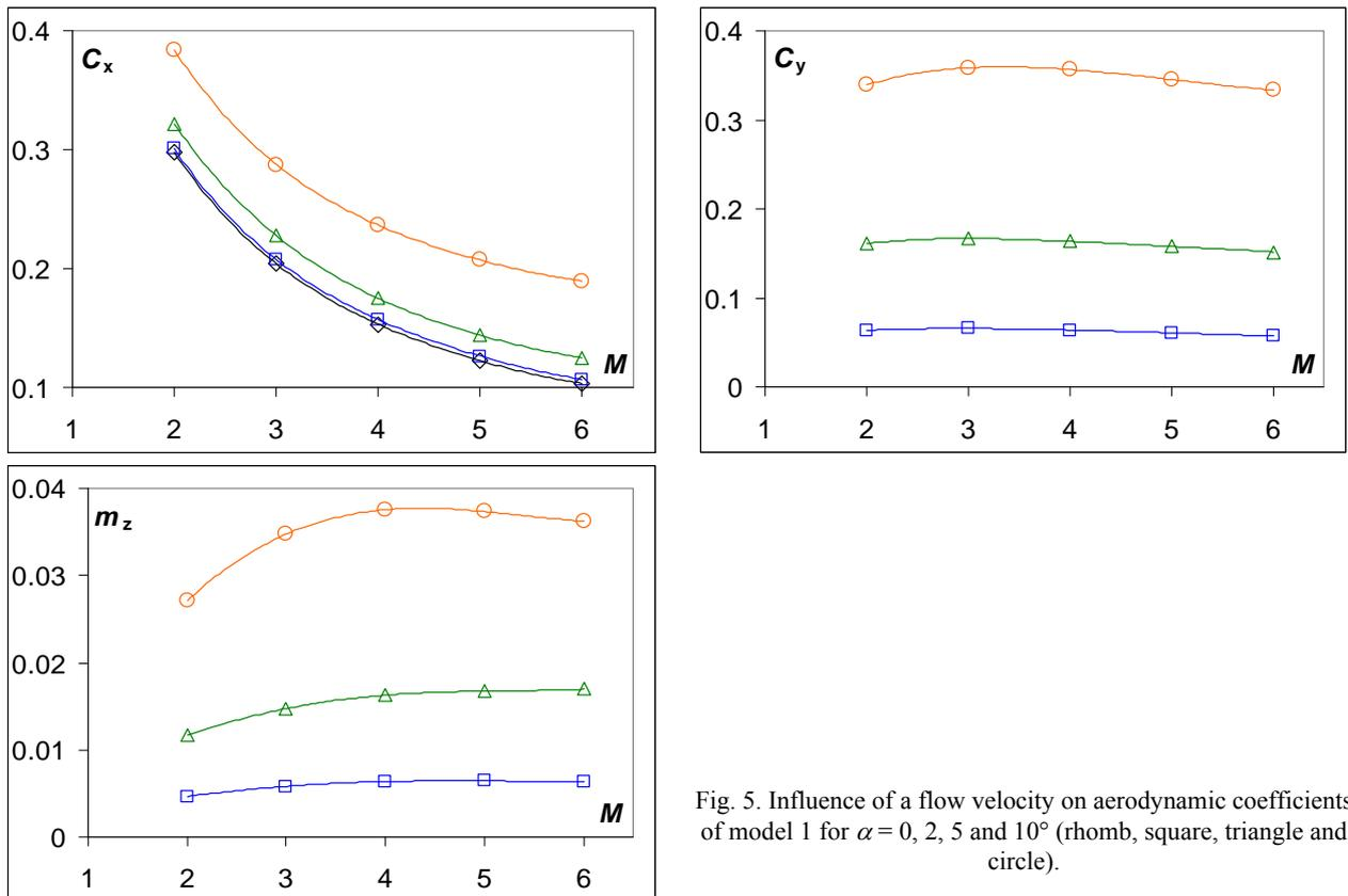
Fig. 5. Influence of a flow velocity on aerodynamic coefficients of model 1 for  $\alpha = 0, 2, 5$  and  $10^\circ$  (rhomb, square, triangle and circle).
