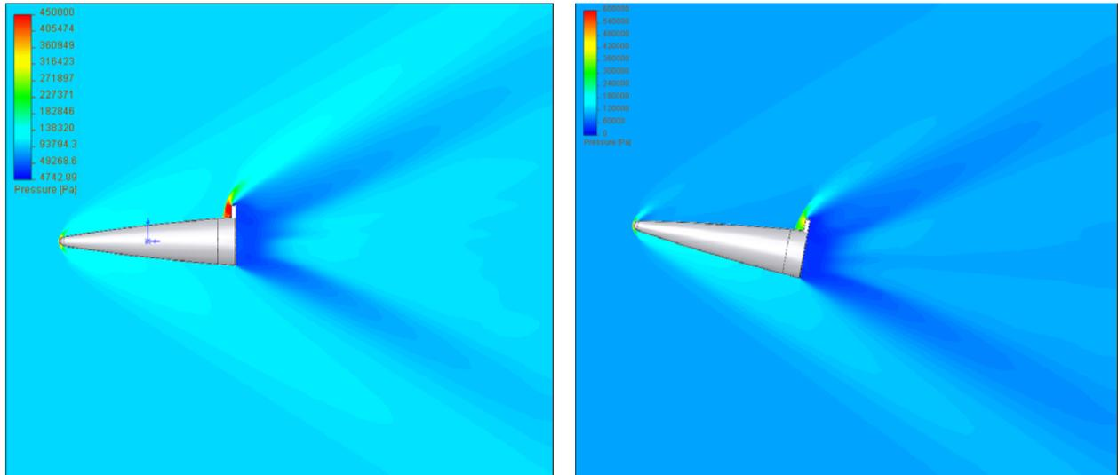
Fig. 9. Flow character of model 3 (pressure fields) for  $\alpha = 0^\circ$  (left),  $\alpha = 10^\circ$  (right) and  $M = 2$ .
