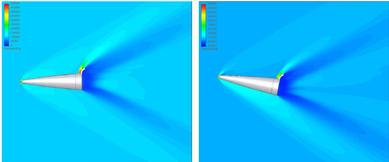
Fig. 12. Flow character of model 4 (pressure fields) for  $\alpha = 0^\circ$  (left),  $\alpha = 10^\circ$  (right) and  $M = 2$ .
