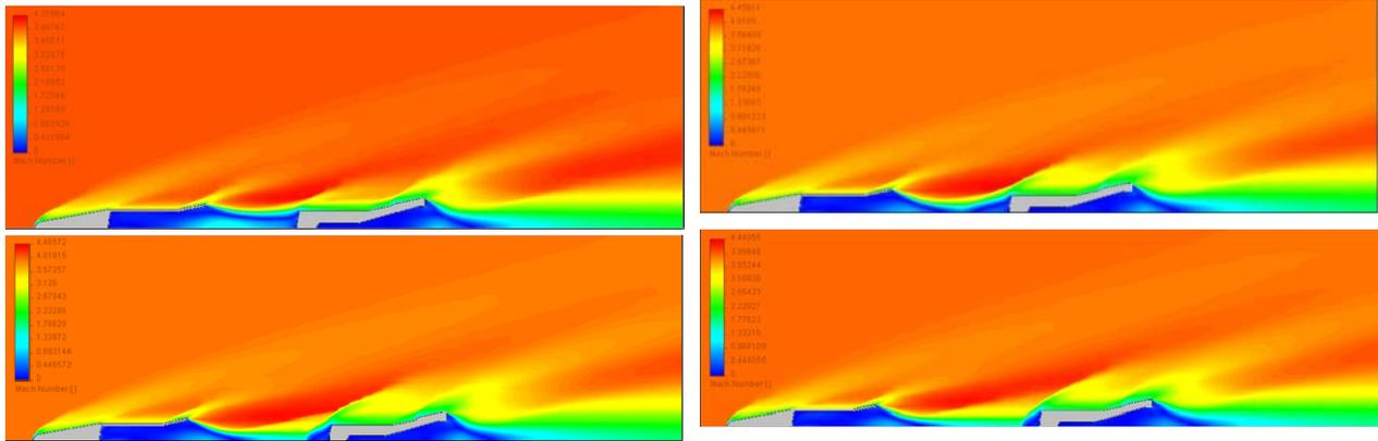
Fig. 18. Joint flow character (Mach number fields) of the leader and block situated at a different distance ( $\Delta = 0, 1, 1.5, 2, 2.5, 3D$  – left to right, top to bottom) at a flow velocity corresponding to  $M = 4$ .
