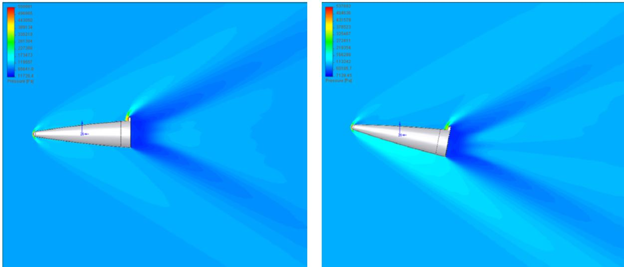
Fig. 6. Flow character of model 2 (pressure fields) for  $\alpha = 0^\circ$  (left),  $\alpha = 10^\circ$  (right) and  $M = 2$ .
