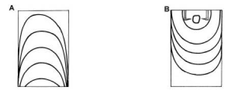
Fig. 11. History of flame propagation in the propane/air mixture with a concentration of 2.25% C<sub>3</sub>H<sub>8</sub> under normal gravity (A) and microgravity (B) conditions. Points of ignition shown in Fig. 3. Flame propagation is indicated in the form of its successive contours. Distance between subsequent contours equal to 8 frames. Frame rate: 250 frames/s
