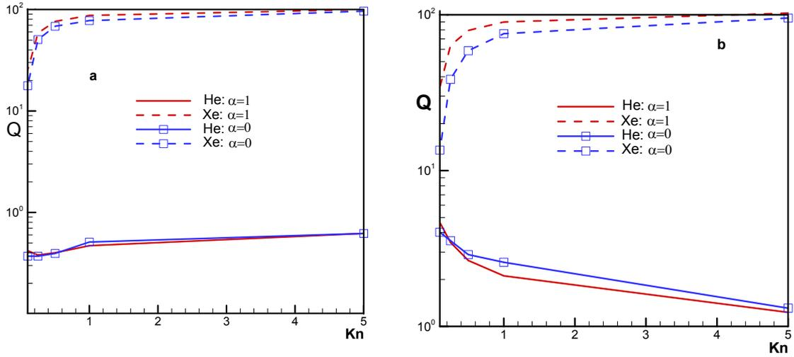
**FIGURE 4.** Dependences of heat flux on the Knudsen number  $Kn$  for Xe (dashed line) and He (solid line).  $\Theta=0.01$  (a) and  $\Theta=0.1$  (b).  $T_w/T_S=9.33$
