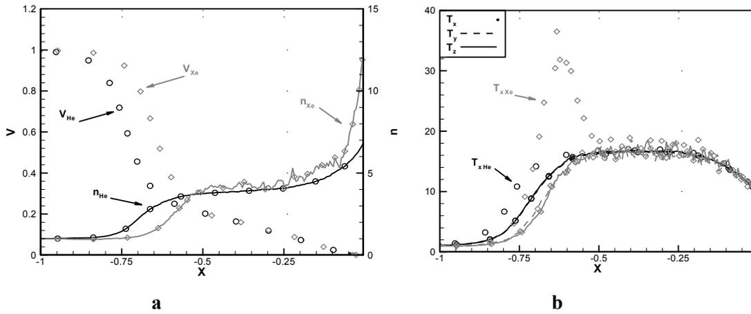
**FIGURE 7.** Density (a) and temperature (b) profiles for small Knudsen number.  $Kn=0.01$ ;  $T_w/T_S=9.33$ ;  $\Theta^{Xe} = 0.03$ .
