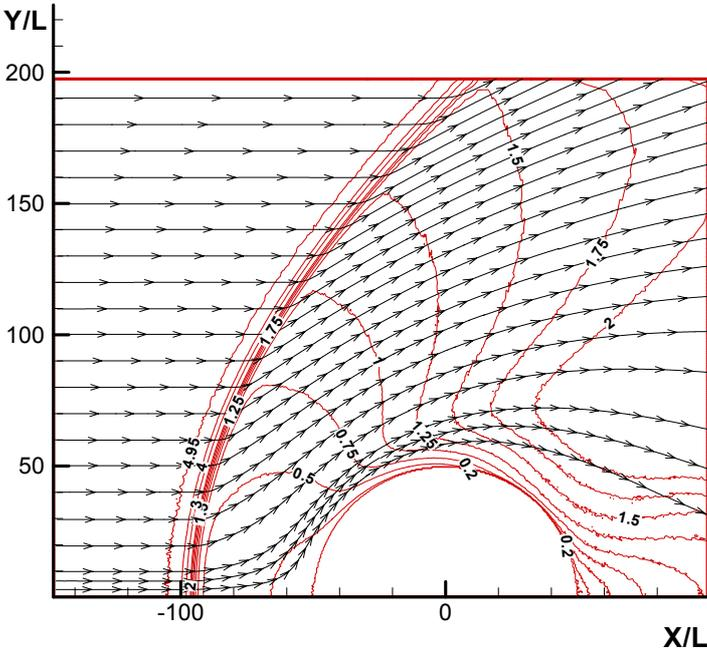
**FIGURE 1.** Streamlines and Mach number contours for pure helium ( $\Theta = 0$ ) at the Knudsen number of 0.01.
