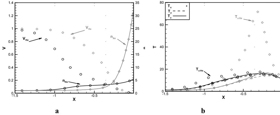
**FIGURE 8.** The changing of velocities and densities (a) and temperatures (b) in the front of the band at  $Kn=0.1$ ;  $T_w/T_s=10$ ;  $\Theta^{Xe} = 0.03$  without xenon absorption.
