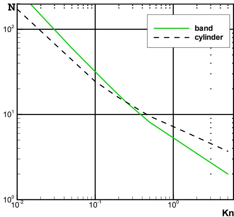
**FIGURE 6.** Helium mean free path number in the shock wave and the compressed layer at  $T_w/T_s = 9.33$ .
