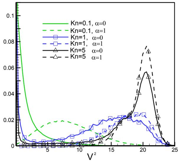
**FIGURE 5.** Distribution function of  $V^2$  xenon atoms colliding with the cylinder for different Knudsen numbers and absorption probabilities  $\alpha$ .  $\Theta=0.1$ .
