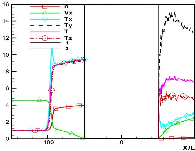
**FIGURE 2.** Distribution of density  $n$ , velocity  $V_x$ , temperature in directions  $T_x$ ,  $T_y$ ,  $T_z$ , and average temperature  $T$  along the plane of symmetry for  $Kn = 0.01$  at  $T_w/T_s=9.33$  for flow of pure helium. Lines 1 and 2 show the size of the cylinder.
