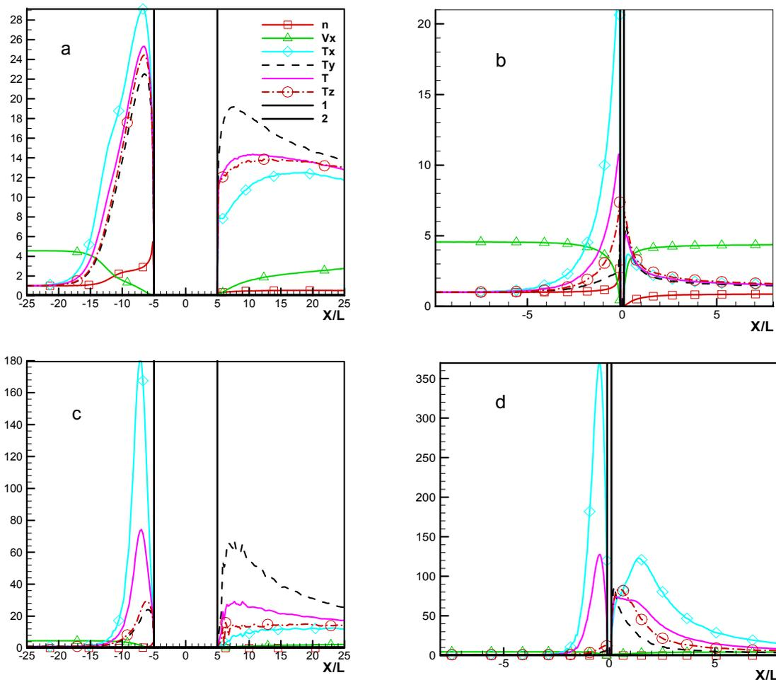
**FIGURE 3.** Distribution for He (a,b) and Xe (c,d) of density  $n$ , velocity  $V_x$ , temperature in directions  $T_x$ ,  $T_y$ ,  $T_z$ , and average temperature  $T$  along the plane of symmetry for  $Kn = 0.1$  (left) and  $5$  (right) at  $T_w/T_s=9.33$ ,  $\alpha=0$  for the flow of gas mixture  $\Theta=0.1$ . Lines 1 and 2 show the size of the cylinder.
