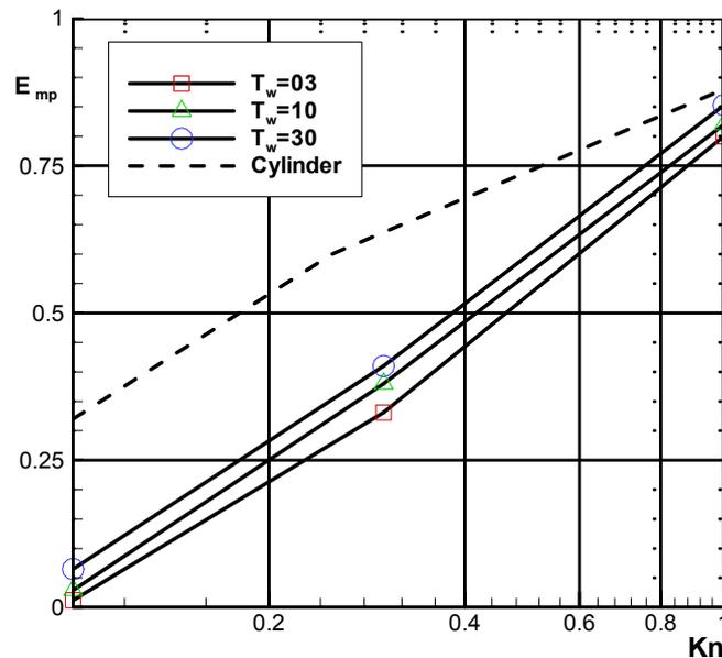
**FIGURE 11.** Dependence of most probable Xe energy  $E_{mp}$  on Knudsen number at different band temperatures ( $\Theta^{Xe} = 0.03$ )(solid lines) and cylinder ( $\Theta = 0.1$ ,  $T_w/T_s=9.33$ ) (dashed line) .
