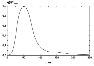
Fig.2 Laser intensity-time profile assumed in the model.
