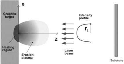
Figure 1. The geometrical scheme of pulsed laser deposition.
