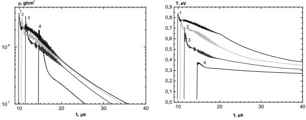
Fig. 5 Calculated carbon plasma density (a) and temperature near the substrate (b) vs. time for energy of the laser pulse: 1 - 10; 2 - 8; 3 - 6; 4 - 4 J.
