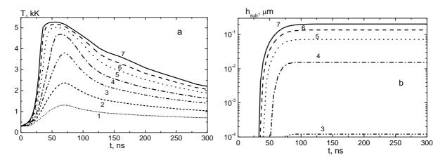
Fig. 3. Calculated temperature at the target surface (a) and evaporation depth (d) vs. time for pulse laser energy: 1 - 1 (6.5), 2 - 2 (13), 3 - 3 (20), 4 - 4 (26), 5 - 6 (40), 6 - 8 (52), 7 - 10 J (65.5 MW/cm<sup>2</sup>). Maximum irradiance is given in brackets.
