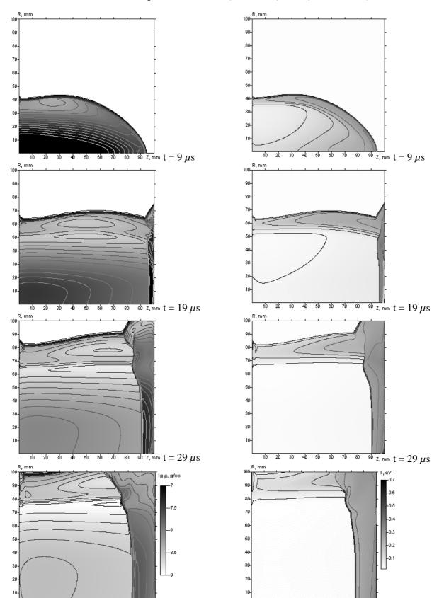
Fig. 4 Carbon plume expansion. Energy of the laser pulse 10 J. Distribution of the density (a) and temperature (b).
