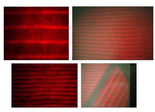
Fig.1. Examples of acoustical standing waves visualized by digital dynamic laser speckle photography
