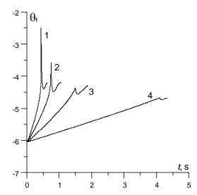
Fig. 3. The film temperature vs. time for different heating rates in the thermal explosion regime for  $\chi$ =0.1 (75 binary layers with the interdiffusion coefficient taken from Ref. [6]). The heating rates are 339 K/s (curve 1), 203 K/s (2), 102 K/s (3) and 33.9 K/s (4)
