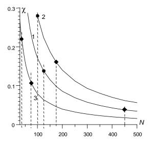
Fig. 2. Parameter  $\chi$  vs. the amount of binary layers in a Ni/Al film on a glass substrate. Numbers at curves correspond to different values of the interdiffusion coefficient: 1, Ref.[4]; 2, Ref.[5]; 3, Ref.[6]. Rhombs denote the limits of SHS for initial temperature 300 °C and circles for 450 °C
