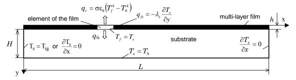
Fig. 1. Sketch of computational region and boundary conditions for the energy transfer equations
