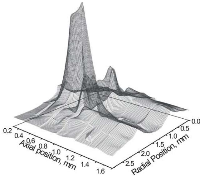
Fig. 2. A picture of radiation of the streamer's head, restored on lateral views of radiation in different sections of the streamer's head. P=740 torr U=30 kV
