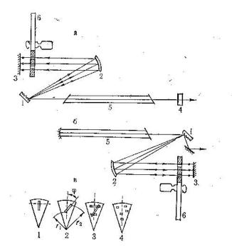
Fig. 2. Different schemes of Soloukhin-Jakoby laser spectrograph
