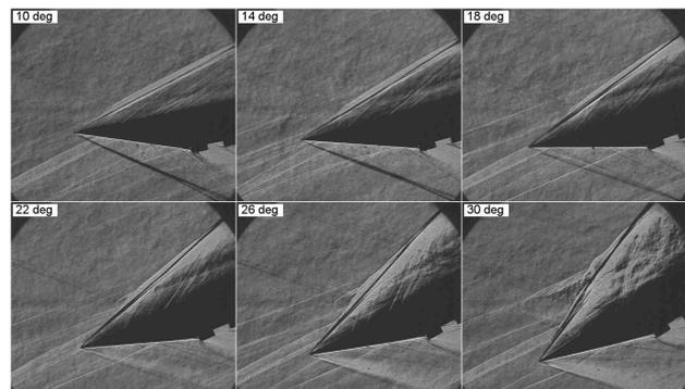
Fig. 2. Vortex / oblique shock interaction at Mach number of 3 and wing angle of attack 10 degrees depending on shock intensity.
