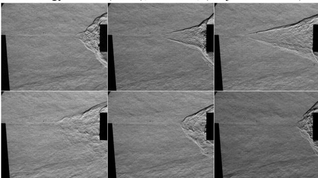
Fig. 1. Different phases of self-oscillations during vortex / bow shock interaction at Mach number of 6 and wing angle of attack 10 degrees.
