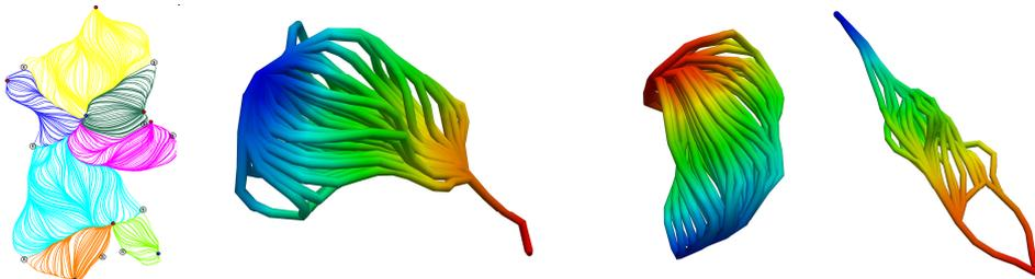
Fig. 1 Schematic illustration of three-dimensional dissipation elements (left) and exemplary dissipation elements obtained from Rayleigh scattering (right).
